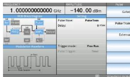
2. Press the F2 soft key to set the Delay of pulse train waveform.
