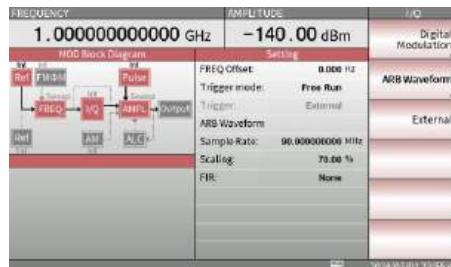
4. To select external waveform modulation, press the F3 key.
