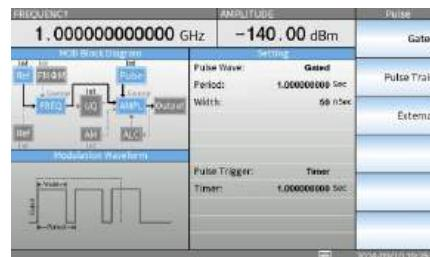
2. Press the F1 soft key and the F2 soft key to set the Gated's Period and Width of the free run waveform respectively.
