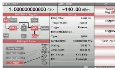
7. Press the F1 key to select polarity. There are polarities positive and negative. You can see the difference from the BNC input route diagram.
