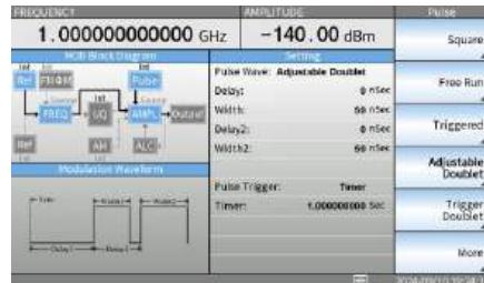
2. Press the F1 soft key, the F2 soft key, the F3 soft key, and the F4 soft key to set the Delay, Width, Delay 2, and Width 2 of the adjustable doublet waveform, respectively.
