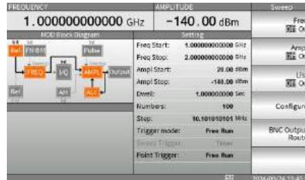
2. Press the F1 key to activate sweep frequency. Then you will see sweep frequency is activated in the MOD Block Diagram and present sweep frequency, as shown in the figure below.
