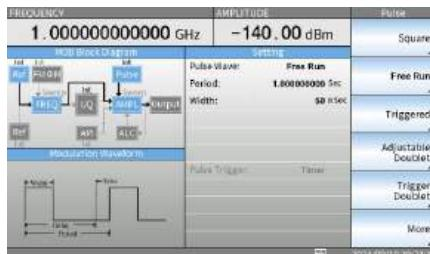
2. Press the F1 soft key and the F2 soft key to set the Period and Width of the free run waveform respectively.
