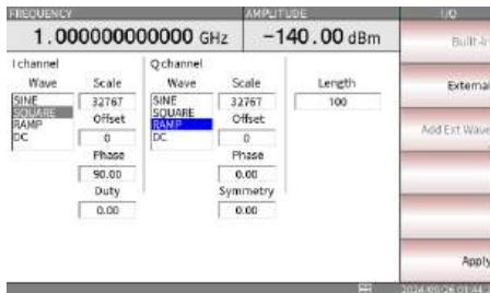
5. Press the F6 key to apply the edited waveform to be inserted.
