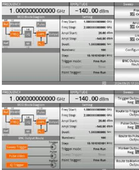
As shown in the diagram below, When the F5 key is pressed, the BNC output route will display on the left lower corner of the Sweep setting page.
