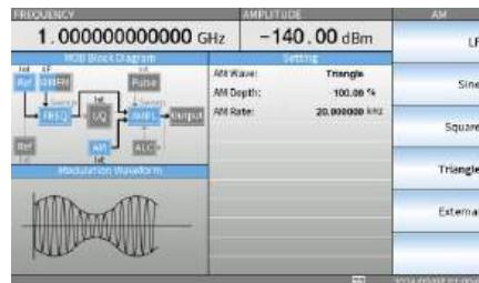
2. Press the F2 soft key to set the AM Depth and press the F3 soft key to set the AM Rate.
