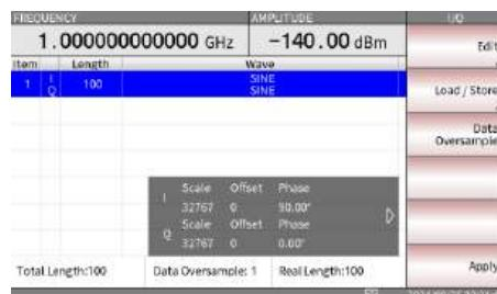
Insert Waveform 3. Press the F1 key to insert a ARB waveform.
