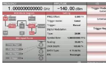
6. To select the External trigger, press the F2 key.
