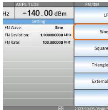
3. After selecting the waveform, press the F1 or F2 keys (according to the waveform you selected) for further setting items. For example, if the Sine waveform is selected, press the F1 key to set Deviation and press the F2 key to set Rate.
