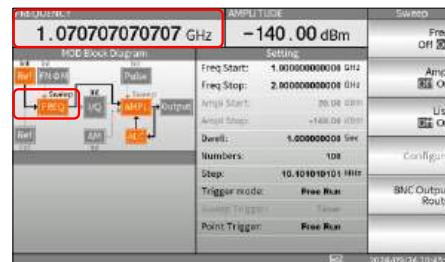
3. Press the F2 key to activate sweep amplitude. Then you will see sweep amplitude is activated in the MOD Block Diagram and present sweep amplitude, as shown in the figure below.
