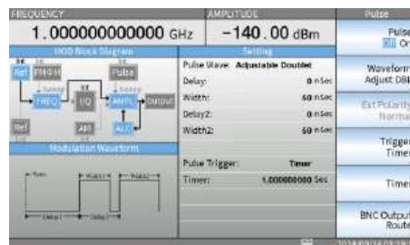
2. To set the pulse trigger to a Timer, Press the F1 key.
