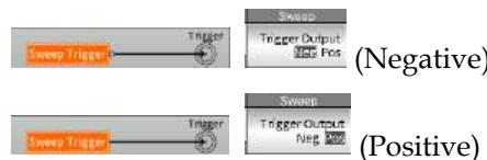
3. Press the F2 key to select which kind of route to trigger output. There are five types of routes available including Pulse Video, Pulse Trigger, Sweep Trigger, Sweep Run, and IQ Generator Trigger.
