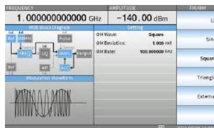
2. Press the F1 soft key to set the  $\Phi M$  Deviation and press the F2 soft key to set the  $\Phi M$  Rate.
