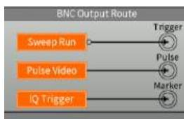
2. Press the F1 key to select the polarity of the trigger output and toggle between Pos and Neg polarity. If Neg is selected, you will see a small icon that looks like a small circle at the end of the route to indicate that the present output polarity is Negative.
