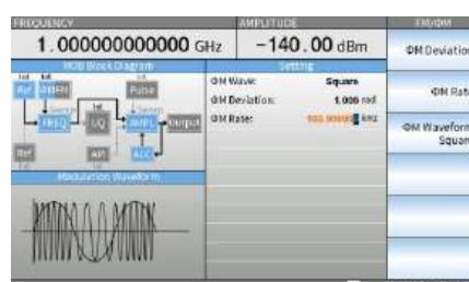
3. Set the value of  $\Phi M$  Deviation and  $\Phi M$  Rate.
