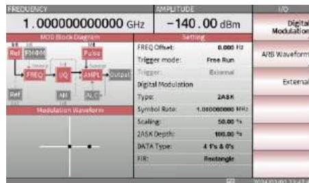
3. To select ARB waveform modulation, press the F2 key. Then you will see the further option about ARB waveform appears as shown in the figure below. For further ARB waveform settings, please refer to page 138.
