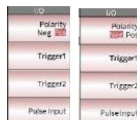
8. Press the F2, F3 or F4 key to select a trigger terminal. Select Trigger 1, Trigger2 or Pulse Input. You can observe which trigger terminal is selected from the BNC input route diagram.
