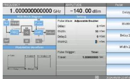
3. Set the value of Delay, Width, Delay 2 and Width 2.
