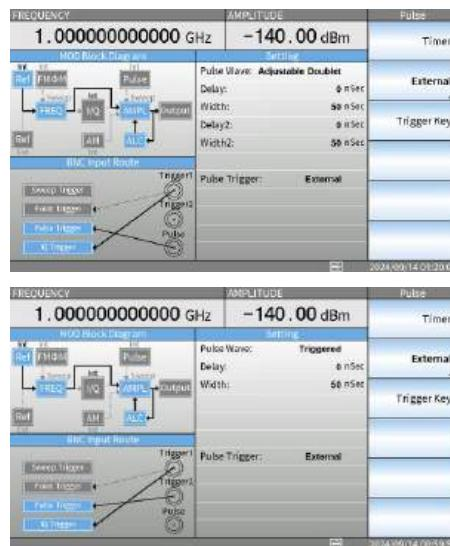
6. Press the F1 key to select polarity. There are polarities positive and negative. You can see the difference from the BNC input route diagram.
