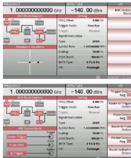
When the F1 key is pressed, the BNC output route will display on the left lower corner of the I/Q setting page as shown in the diagram below.
