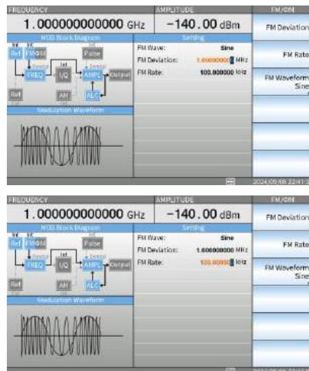
4. Use the left and right arrow keys to select the digit to be changed and then use the up and down arrow keys to increase or decrease the value of the digit to be edited.
