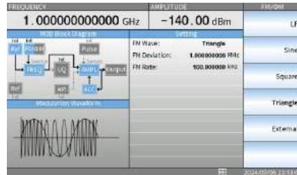
2. Press the F1 soft key to set the FM Deviation and press the F2 soft key to set the FM Rate.
