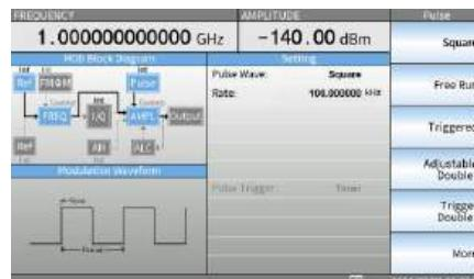
2. Press the F1 soft key to set the Rate of square waveform.
