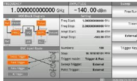
6. Press the F1 key to select polarity. There are polarities positive and negative. You can see the difference from the BNC input route diagram.
