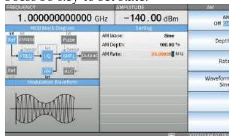
5. Use the left and right arrow keys to select the digit to be changed and then use the up and down arrow keys to increase or decrease the value of the digit to be edited.
