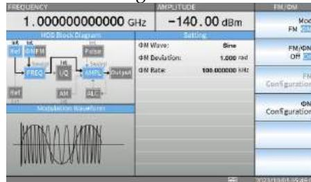
8. To change the FM modulation waveform, press the F3 key and select a wave you need. The following steps for changing waveform is similar to those indicated above in step 2 through step 6.
