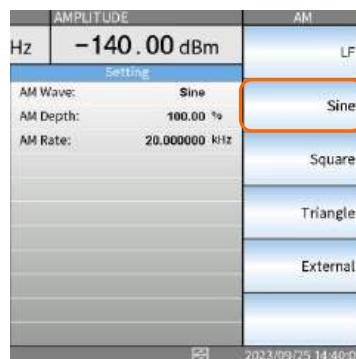
2. Configure the setting of wave form that has been selected. For example, if "Sine" is selected, you need to configure Depth or Rate of "Sine" wave.
