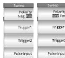
7. Press the F2, F3 or F4 key to select a trigger terminal. Select Trigger1, Trigger2 or Pulse Input. You can observe which trigger terminal is selected from the BNC input route diagram.
