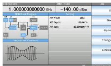
2. Press the F2 soft key to set the AM Depth and press the F3 soft key to set the AM Rate.
